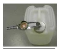
Step 4. Torque the cap to 150-160 in-lbs.
